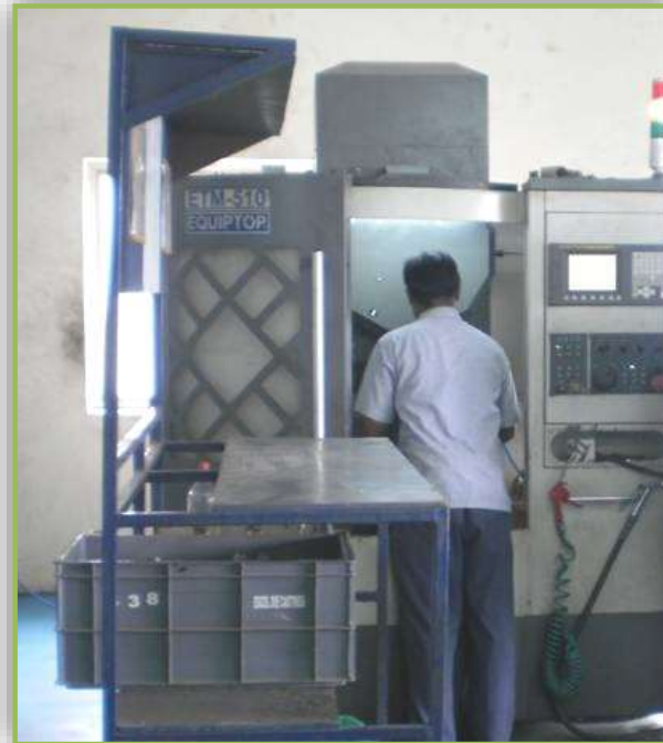
VMC Machine EQUIPTOP TAIWAN ETM-510 BED SIZE (600 X 360)MM
